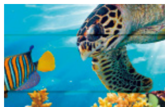
Overlap/Black streaks (Insufficient feeding amount)
